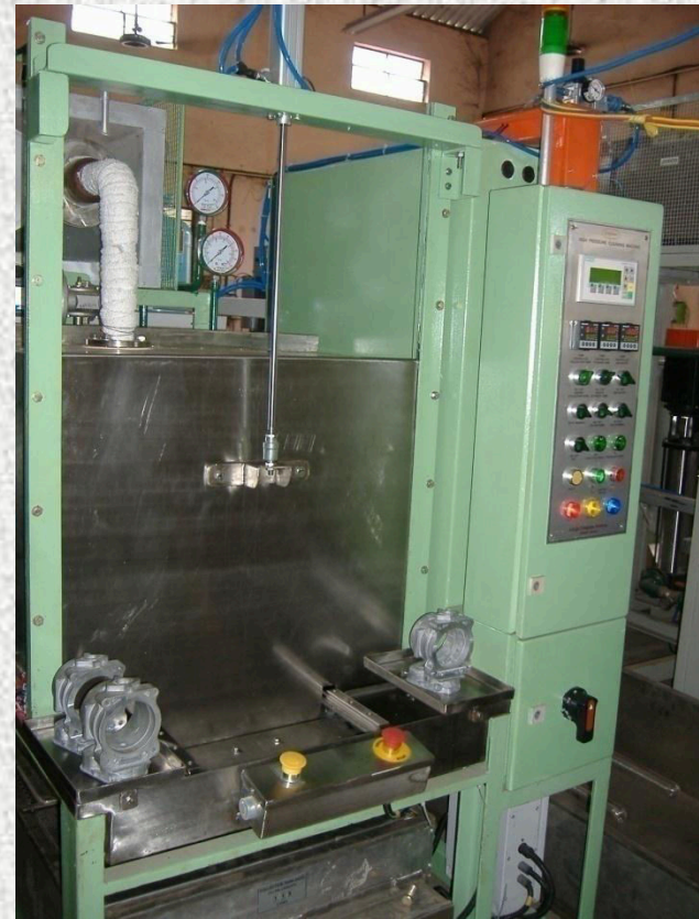
SHUTTLE TYPE WASH < RINSE AND HOT AIR DRY MACHINE FOR BATCH PRODUCTION
